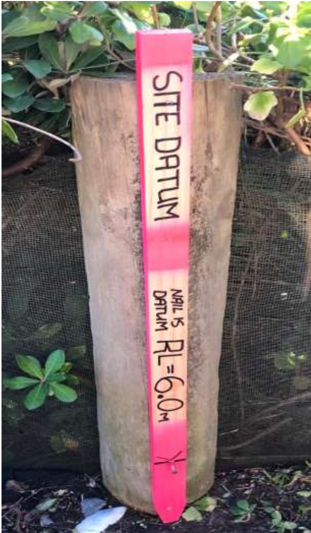
Surveyor's mark at 7 Marine Parade Otaki Beach showing the land being 6 metres above mean sea level.
